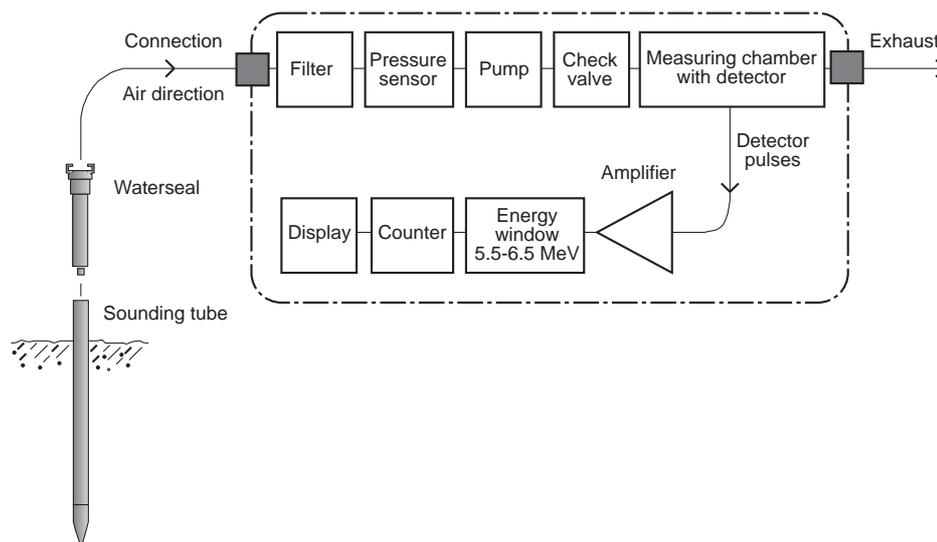
In the initial measuring phase, air from the soil is pumped up through the sounding tube into the measuring cell. The pumping time (about 30 sec) has been chosen to ensure that all fresh air in the system is pumped out.
